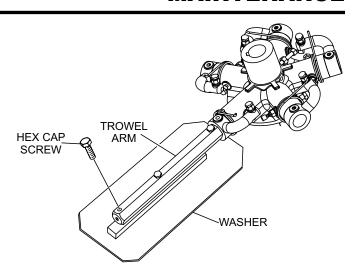
Figure 33. Blade Removal
